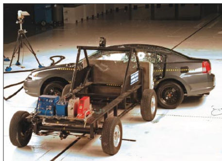
Highway Safety Committee members witnessed the controlled crash of a 2004 Mitsubishi Galant at the Insurance Institute for Highway Safety. The crash was a 50 km/h side impact that simulated a collision between the sedan and a sport utility vehicle.
