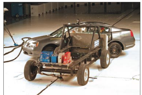
Highway Safety Committee members witnessed the controlled crash of a 2004 Mitsubishi Galant at the Insurance Institute for Highway Safety. The crash was a 50 km/h side impact that simulated a collision between the sedan and a sport utility vehicle.
