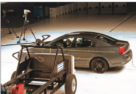
Highway Safety Committee members witnessed the controlled crash of a 2004 Mitsubishi Galant at the Insurance Institute for Highway Safety. The crash was a 50 km/h side impact that simulated a collision between the sedan and a sport utility vehicle.
